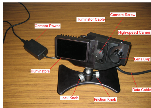
Figure 3-5: Parts of the EyeLink 1000 Desktop Mount
