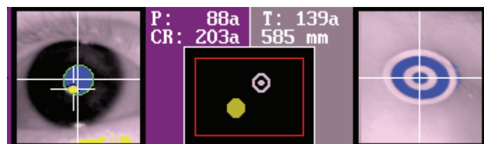
Figure 3-12. Target and Eye Positions in the Thumbnail Camera Images
