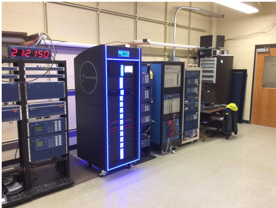
Fig. 1: UI RTDS with protection and control hardware
