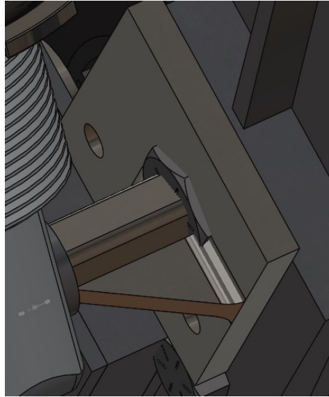
Figure 18: View of forward suspension arm's shock mount. Mounts forward shock to left runner intermediate axle mounting plate
