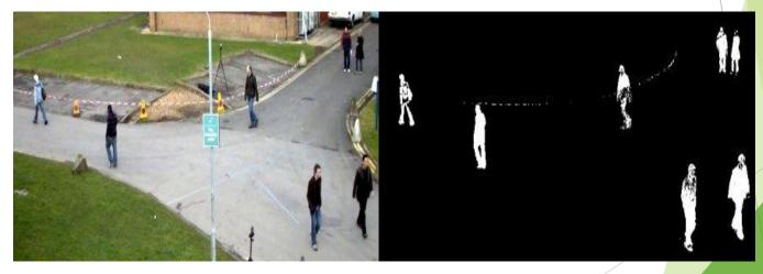
A theoretical example of an image OpenCV would end up with to do motion detection.
