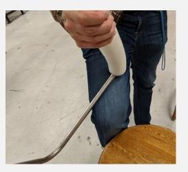
Going into the second 90° bend, there is already a need for a third point of contact on the tube assisting the insulation process.
