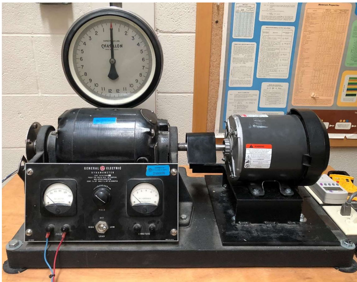
Fig. 1. Dynamometer on the left, Asynchronous motor on right and scale is above dyno. This is the initial set up of the dyno before disconnecting the current motor and mounting the TG5153 frame.
