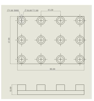
Screw holder with set screw locations. We ended up needing to use set screw locations because the screw delivery system ended up being more advanced than expected. The diameter of the holes are about 2 mm larger than the screws. This allows the screws to be picked up without resistance from the holder while still being tight enough to not allow the screw to move around too much and able to get out of position to be picked up.
