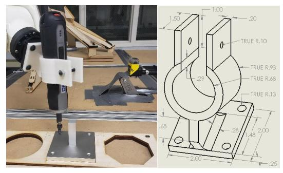
Updated end effector for for Robot #2. We changed to a clamping end effector because the thumb screws were tearing the rubber on the torque screwdriver and therefore moving the screwdrivers location. Using a clamp fixes this problem
