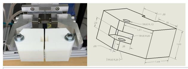
End effector for robot#1. These grippers are air pressurized so they can open and close.
