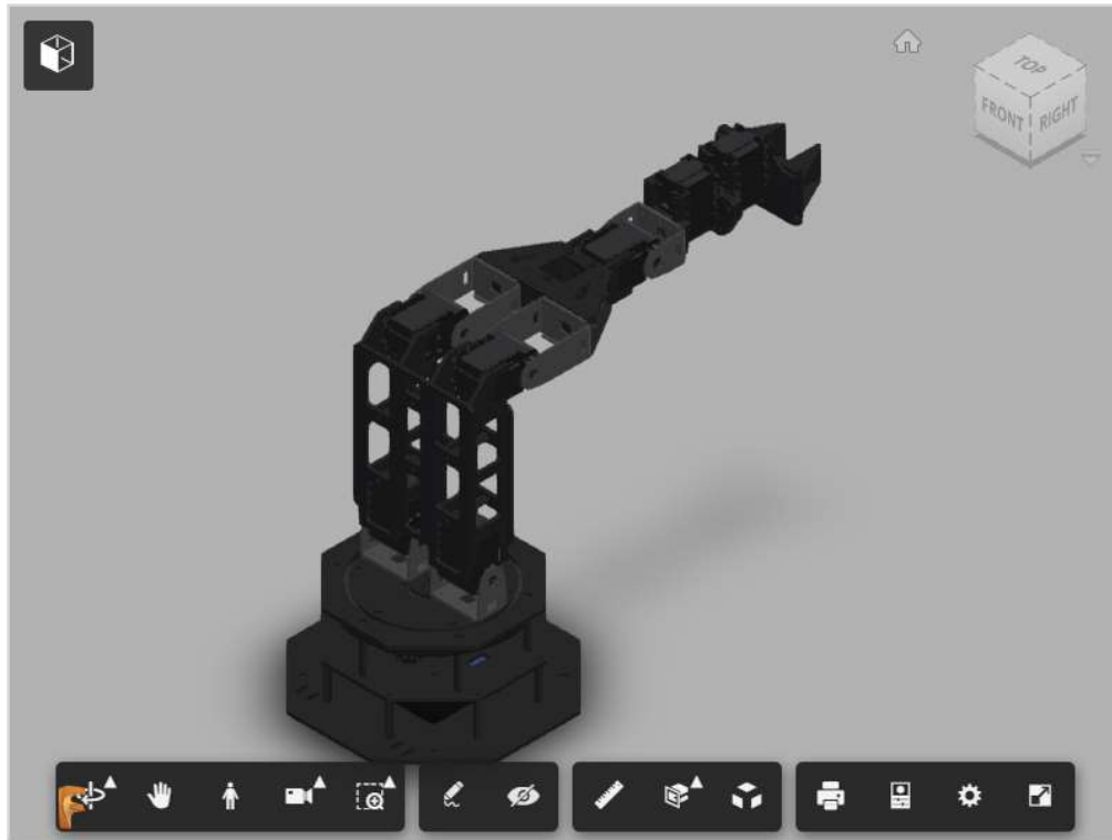
Figure 1: 3D Robot Visualization provided at Trossen Robotics Website . The assembly can be pulled apart, and parts can be measured in any legitimate units system to satisfy any replacement needs.
