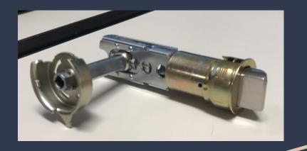
• Use existing door latch assembly to interface with door handle.
