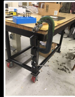
Load testing of ball joints.
