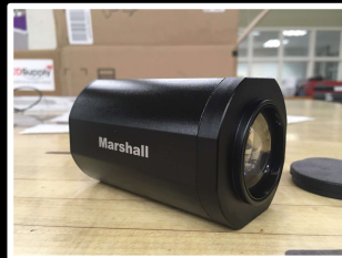
Marshall CV350-10XB, weighs 375g, has a 10X zoom
