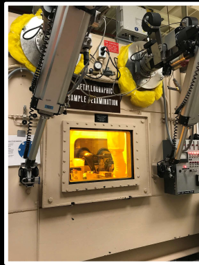
View of operating window in the front of the Met Box.
