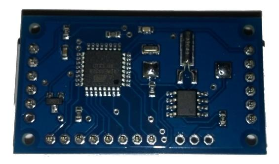
Solder the connectors on. Start with one pin and check to ensure it maintains perpendicular orientation.
