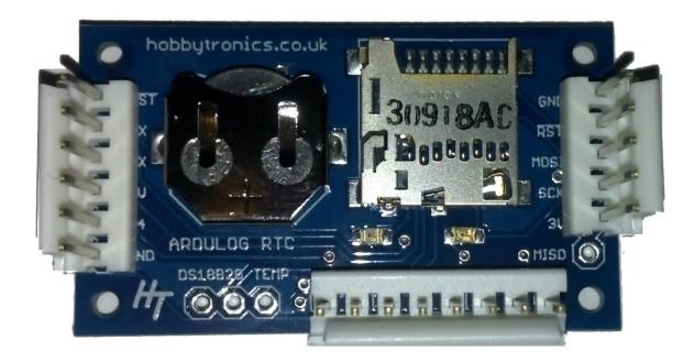
Flip over with leaving the connectors inserted and ensure they are approximately perpendicular to the board.
