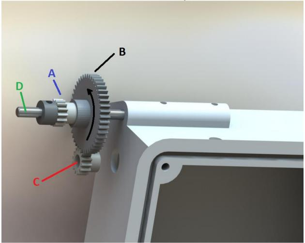
A+B) the 14t and 44t 32pitch delrin gears, fixed to each others rotation by the sleeve bushings underneath
