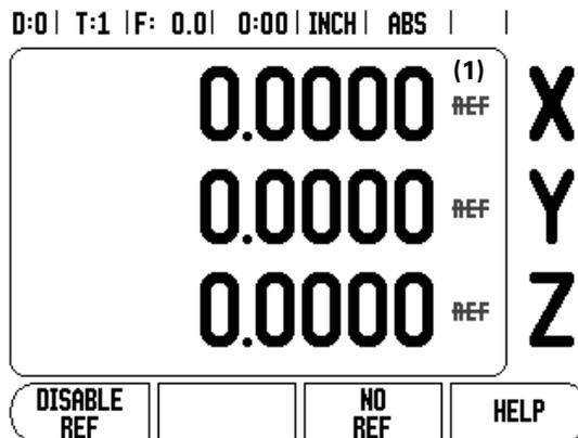
The 200S can still cross over reference marks at a later time. Such as if it becomes necessary to define a datum that can be re-established after a power interruption.
