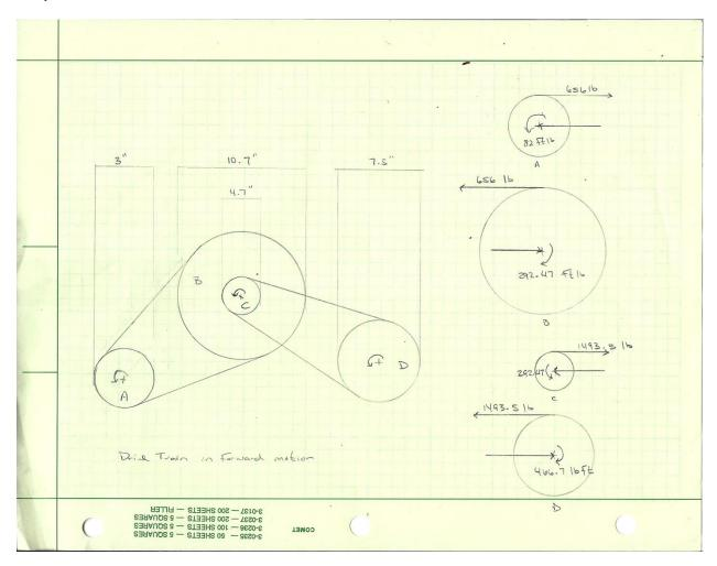
This model helped us determine the output torque at the front driveshaft. This torque was needed to be able to continue the design of the drive shafts and sprocket/chain sizes needed for the rest of the chain drive. It also helps us calculate the torque that the snowmobile should theoretically be putting to the ground (ideal conditions).
