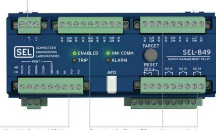
Connectors for the thermistor input and AO let you monitor the equipment temperature and integrate with a distributed control system (DCS).
