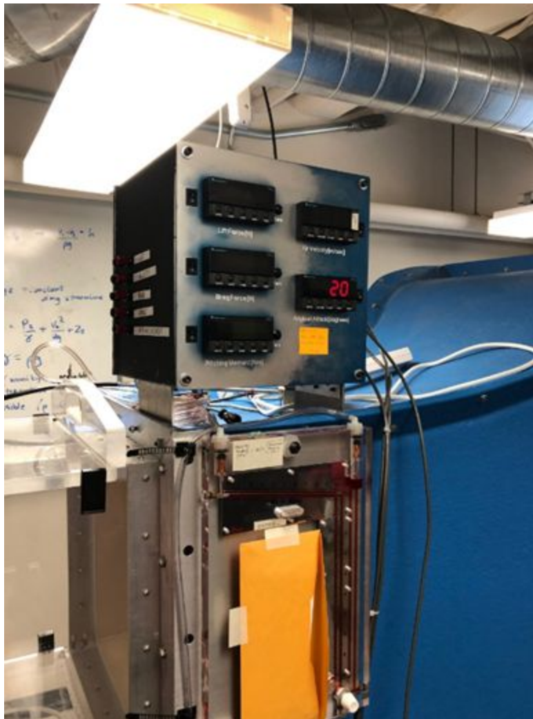
Figure 2. Current data acquisition system that outputs lift force, drag force, pitching moment, velocity, and angle data.
