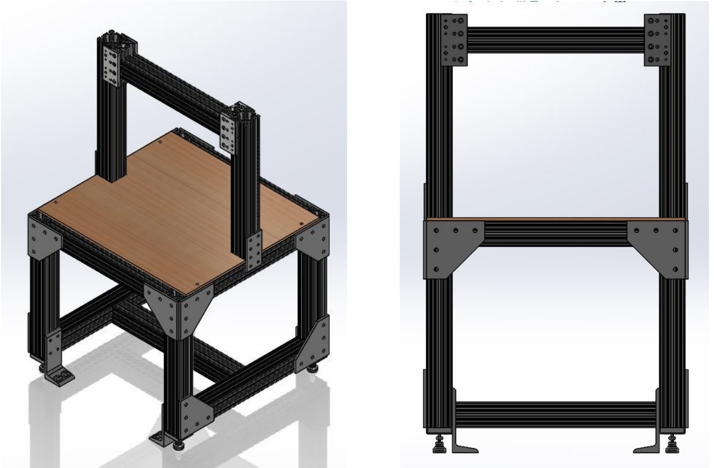
Figures 4 & 5. The left figure (4) shows the final stand that was built. The right figure (5) shows a side view of the stand that emphasizes the upper sliding mechanism.
