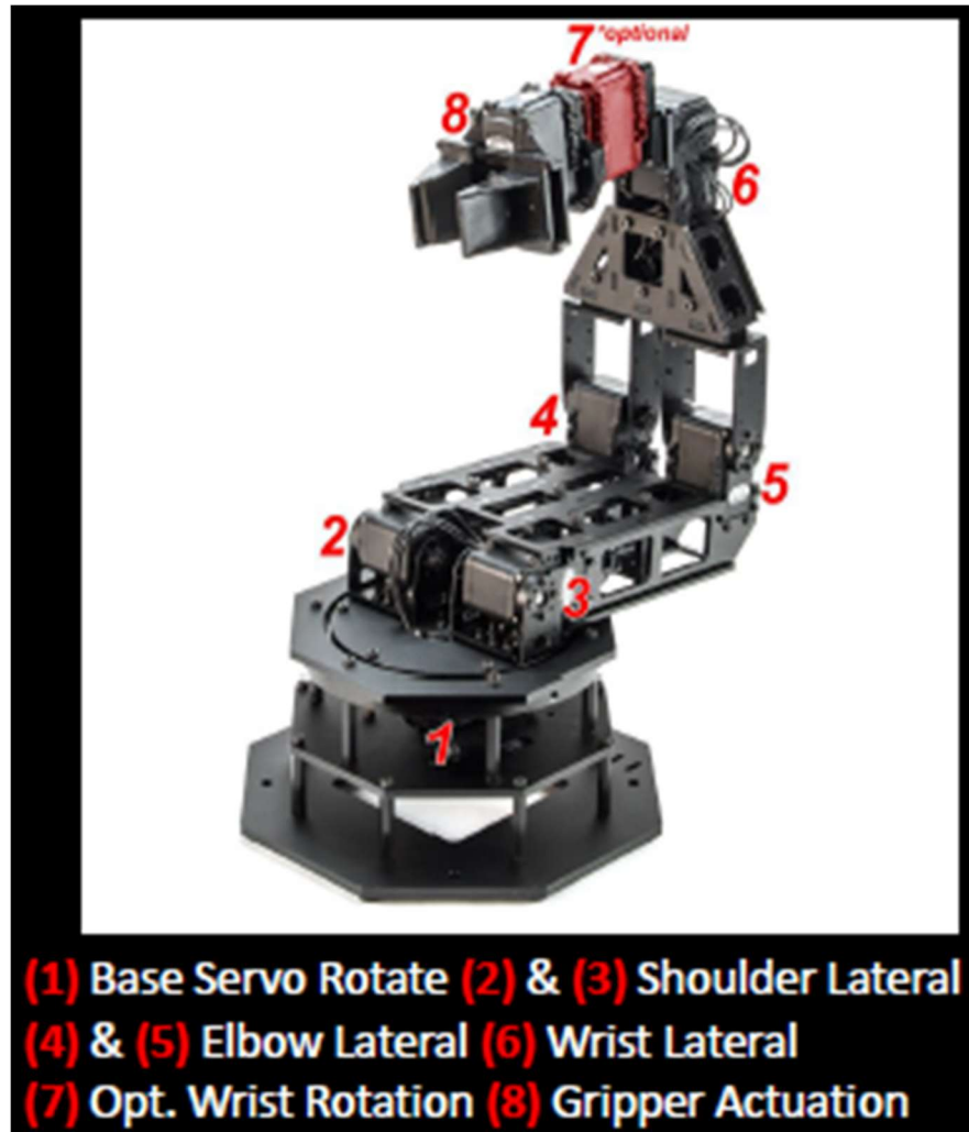
Figure 16: Servo-Motor Diagram depicting the name, and motion of each Servo-Motor.
