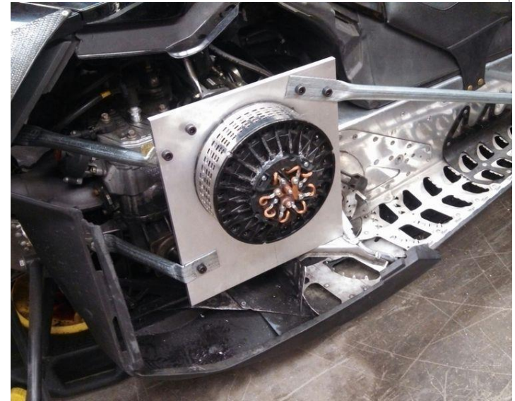
Electric Motor Mount Built for Dyno Testing
