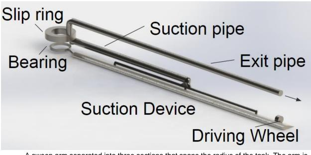
A sweep arm separated into three sections that spans the radius of the tank. The arm is driven by a wheel at its tip and incorporates our slip ring design.
