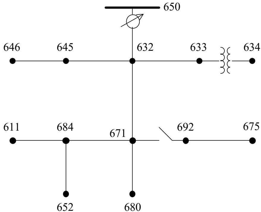
Figure 1 : One-Line Diagram of IEEE 13 Bus Power System [1]
