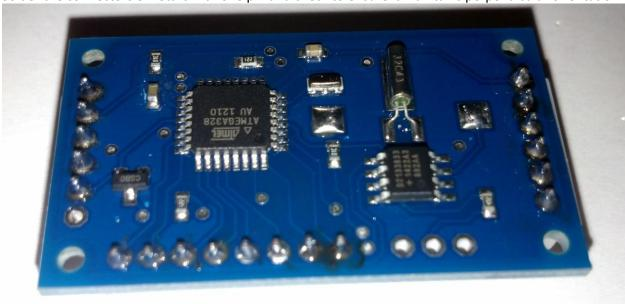
Install the Dallas temperature sensor with the flat part facing outward. Spread the two out leads to keep the device in place. Solder and trim the wires.
