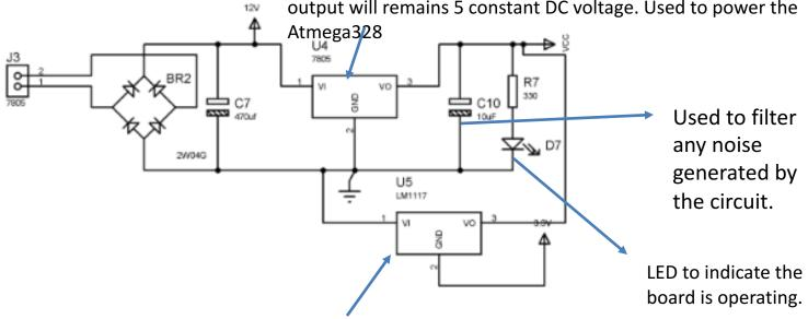
To regulate the 5 DC voltage to 3.3 DC voltage to power the ZigBee.
