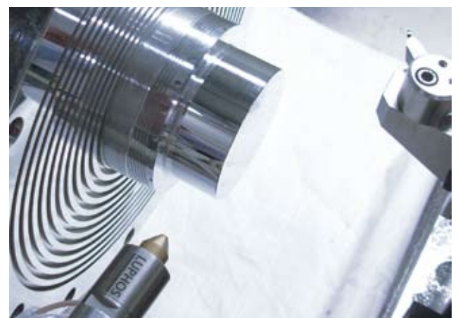
Measuring the concentricity of a diamond turning machine.
