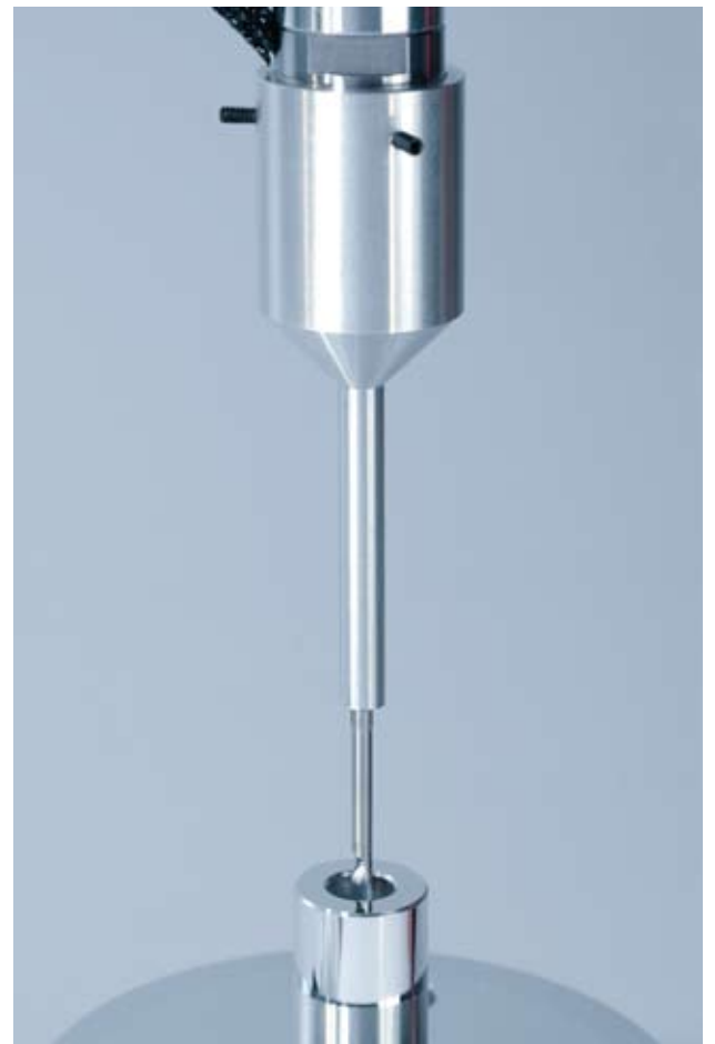
Probe adapter for bore hole measurements.
