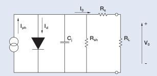
Figure 3. Equivalent Circuit for the silicon photodiode
