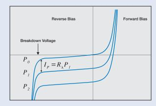
Figure 7. Characteristic I-V Curves of an OSI Optoelectronics photodiode for Photoconductive and Photovoltaic modes of operation. P<sub>a</sub>-P<sub>a</sub> represent different light levels.
