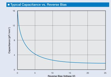
Figure 4. Capacitance of Photoconductive Devices versus Reverse
