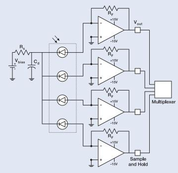
Figure 11. Circuit example for a multi-element, common cathode arrav
