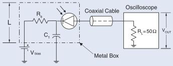
Figure 9. Photoconductive mode of operation circuit example: High Light Level / High Speed Response
