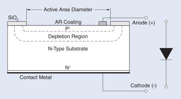
Figure 1. Planar diffused silicon photodiode
