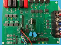
Power converter with voltage and current sensor
