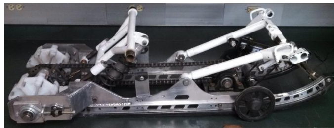
Figure 4. Team Rear Motions chain driven rear drive design
