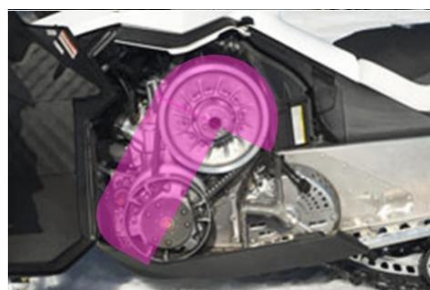
Figure 1. Example of clutch cover and stock brake cover shown from Clean Snowmobile Challenge Competition rules.
