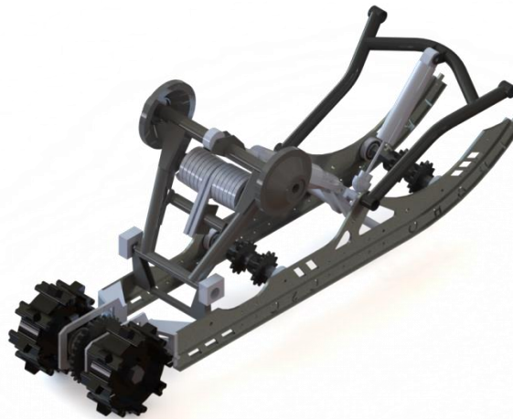
Figure 9. Chain drive conceptual design
