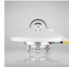
CMP10 Pyranometer Provided by the University of Idaho
