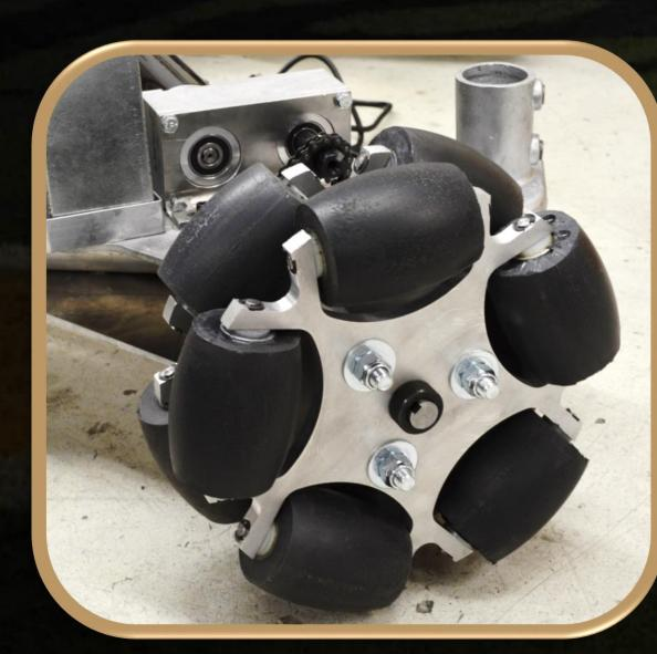
IVIODIIITY Omni wheels for multidirectional movement Custom molded urethane rollers Independently driven wheels with a 24:1 gear reduction
