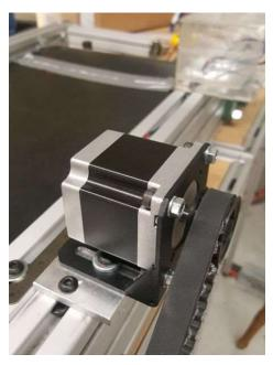
The stepper motor shall be mounted directly onto the conveyor, on the adjustable part, so as to maintain tension in the belt connected to the bearing.
