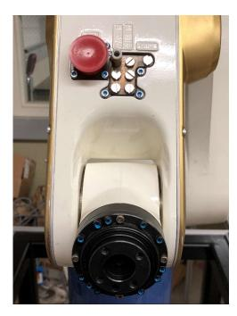
Any electrical or pneumatic connections will be attached into the back of the robotic arm, seen in the figure at the left. If connecting to the tool slot in the arm, the connections above the black screw ring will be used, seen at the right. Any tool must be able to screw into the figure at the right to be able to attach to the arm, which has a square screw fit and 1.266 inch diagonal.
