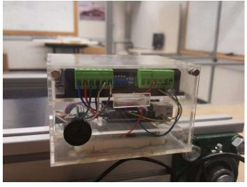
The controller, Arduino, and wiring for the conveyor shall be placed into an acrylic box to avoid any wiring mishaps from the surrounding environment. This box shall be entirely closed, with a removable door in order to replace wiring if deemed a necessity.
