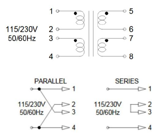
We should connect the primary side of PT to the AC power supply and use multimeter to read values at secondary side, then compare the ratio. Due to the close of power lab, we can not reach the AC power supply.
