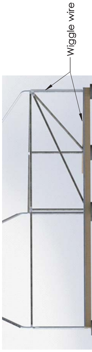
Figure 7: This figure shows how the wiggle wire will mount to the lumber along the windbreak base.
