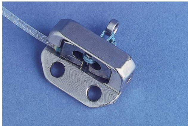
Fig. 2. The assembled sensor as it was implanted into the sheep.
