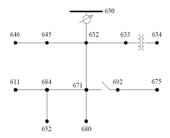
Appendix A –IEEE 13 Node Test Feeder One-Line Diagram
