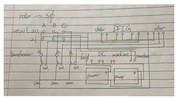
If rotor becomes 3 phase. The frequency of rotor is constant(6Hz). We still can change the field control and field current to change the speed and the frequency of machine, the frequency of stator. We can change the direction of rotation. It also means change the direction of AC voltage.
