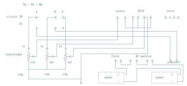
We can change the field current and field control to change the frequency of machine. The frequency of stator is constant. We can change the speed of the machine then know the frequency of machine and rotor.
