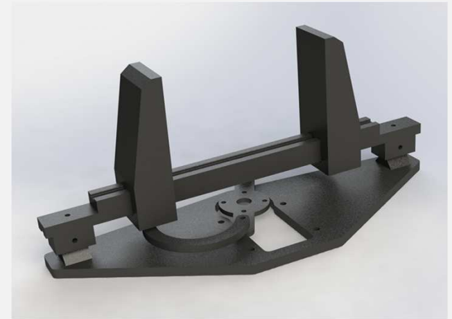
New Gripper can open up to 10 cm wide.
