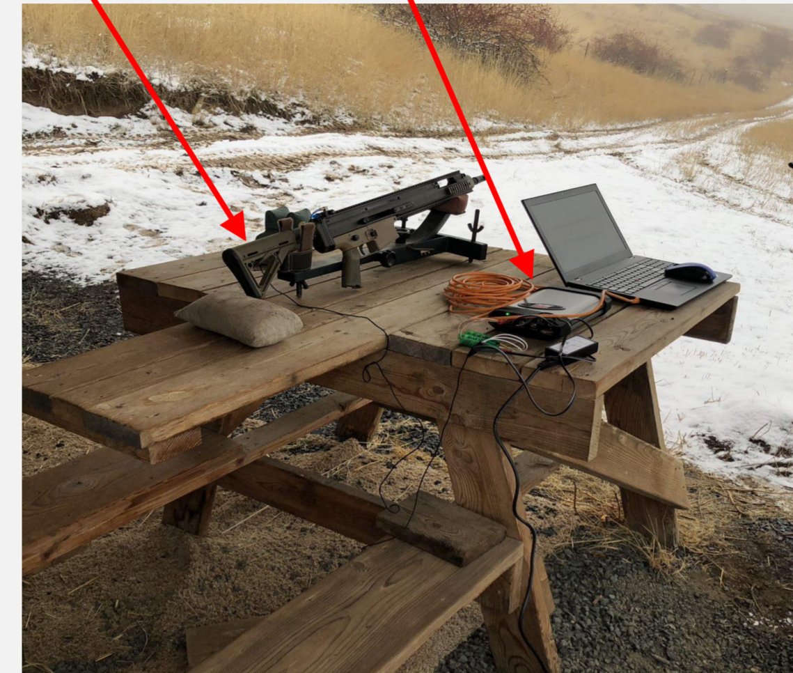
(Left) Live fire setup for acceleration data gathering on mount. (Right) Dytran 3313
