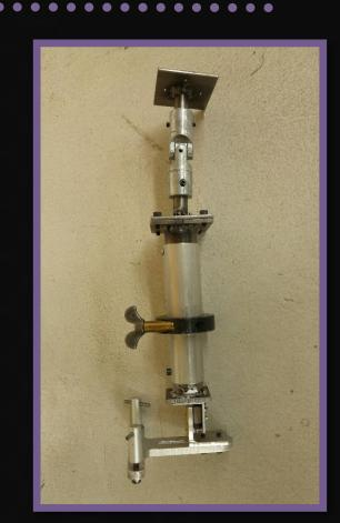
**Pulley Attachment: Convert** vertical force to lateral and mount string potentiometers
