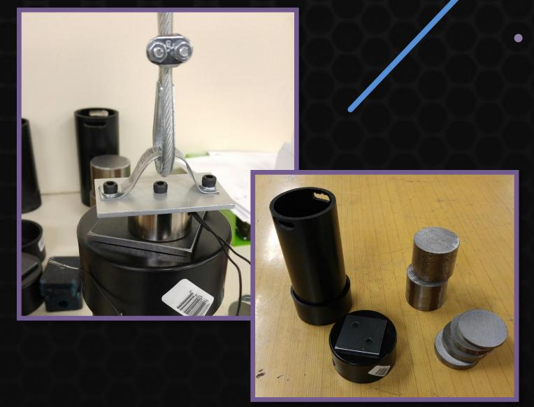
**Torque Arm:** Transmits torsional forces to torque sensor
