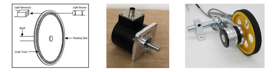
Encoders very accurately measure angles which can easily translate to distance, velocity, and acceleration.
