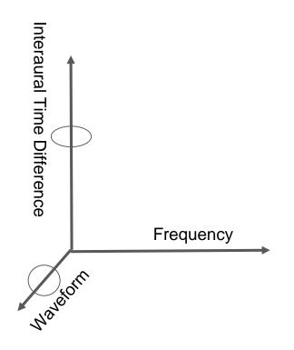
Three spatial dimensions must be mapped to 3 distinguishable sound characteristics for audio transmission. The three characteristics that will be used are waveform, frequency, and interaural time difference.
