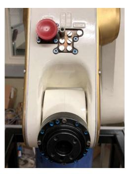
Any electrical or pneumatic connections will be attached into the back of the robotic arm, seen in the figure at the left. If connecting to the tool in the arm, the connections above the black screw ring will be used, seen at the right. Any tool must be able to screw into the figure at the right to be able to attach to the arm.
