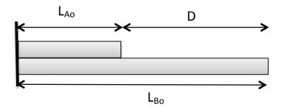
Material A is copper and has a length  $L_{Ao}$  = 1.00 m. Material B is glass. If we want the distance between the ends of the rods, D, to be stable (constant) when the temperature fluctuates, what length  $L_{Bo}$  is needed?
